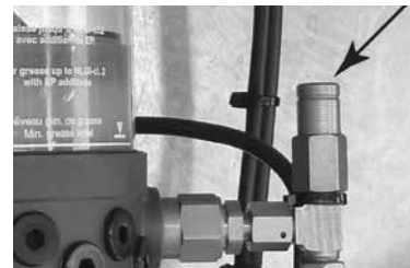
Pressure safety valve
